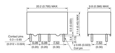
Note The tolerance is  $\pm 0.2$  (0.008) unless otherwise specified. The dimension in the box shows basic size.
